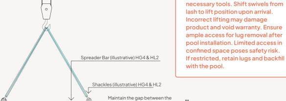
top of the pool and the slings between 50mm and 100mm
